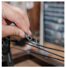
1.6 With the bow string relaxed, remove the wax within a 3 inch area of where the peep will be installed. Mark the spot where the previous peep was embedded before removing the old peep.
