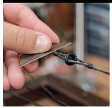
1.1 Use extreme care when removing existing string serving from bow. Bow press must be used. DO NOT use string splitter for this application.
