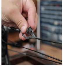
1.4 With the Peep-It posts facing the top cam, Place one side of the peep into the provided grove. Then repeat this process on the other side.
